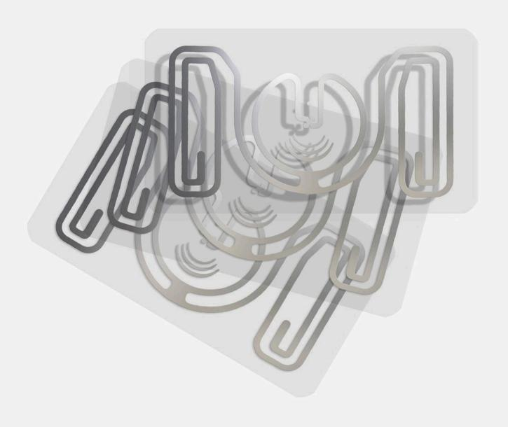
WT002 is a *wet inlay* made of PET. It is flexible, cut- and weather-resistant. Rectangular in shape, it measures 36 mm x 22 mm x 0.23 mm and can be applied to non-metal materials by means of a special adhesive.
