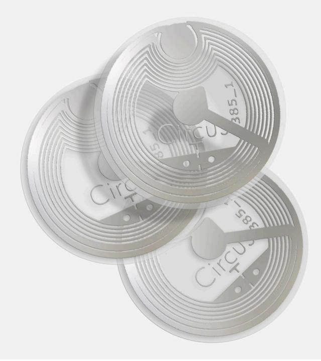
WT004 is a *wet inlay* made of PET, a flexible thermoplastic material resistant to cuts and thermal shock. Round in shape, it has a **diameter of 22 mm and a thickness of 0.2 mm**. It is transparent and is applied to **non-metal surfaces** by means of a special adhesive.
