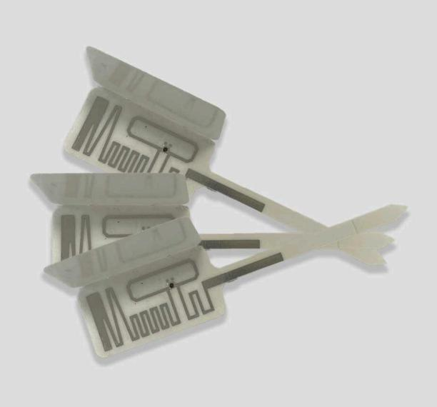
LB032 is an adhesive RFID tag made of PET, rectangular in shape. It measures 64 x 28 mm and operates in the UHF frequency with the MONZA M730 chip. LB032 is applied by adhesive to non-metallic surfaces.
