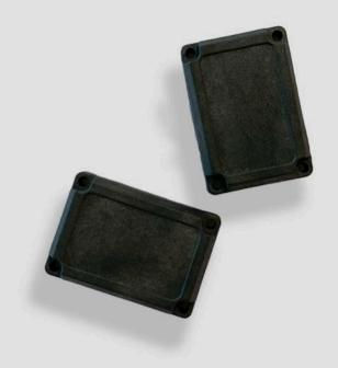
HT072 is an RFID hard tag made of **PEEK**, a thermoplastic material with reduced wear sensitivity, as well as with high impact and high temperature resistance. Rectangular in shape, it **measures 41 x 29 x 9 mm**, weighs 15 grams and can be **screwed** through four holes with a diameter of 2.3 mm **on metal surfaces**.
