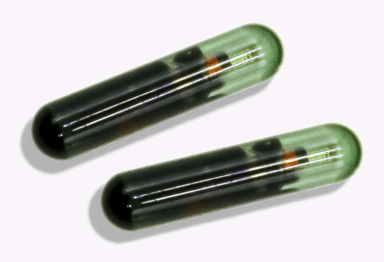
GT002 is a 'glass tag', thus made of glass, a transparent, chemically stable and versatile material. Cylindrical in shape, it is available in two sizes: Ø 2.12 mm x 12 mm and Ø 3 mm x 13 mm. This small size allows the tag to be easily embedded in any surface, whether metal or non-metal (plastic, wood, paper, water). Furthermore, the high resistance of glass protects the electronic components from exposure to aggressive chemicals, ensuring that readability remains
