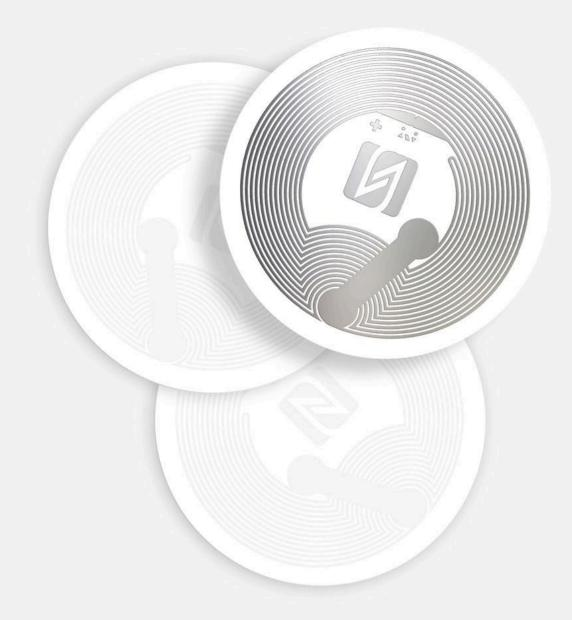
LB004 is a flexible and adhesive paper RFID label. Round in shape, it has a diameter of 40 mm, 0.27-mm thickness, and is designed for application on non-metal surfaces. Printing and serial numbering are applied using offset or inkjet technology for colour and black-and-white prints, and thermographic printing for black-and-white prints.
