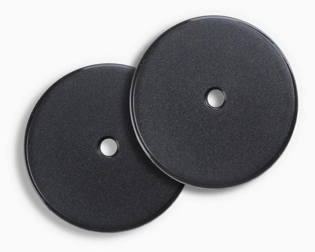
HT001 is an RFID hard tag made of PPA (polyphthalamide), a thermoplastic material with a high resistance to chemicals, moisture and very high temperatures. It also possesses good mechanical properties, which ensure excellent dimensional stability and high resistance to breakage and deformation. With its IP69 rating,
