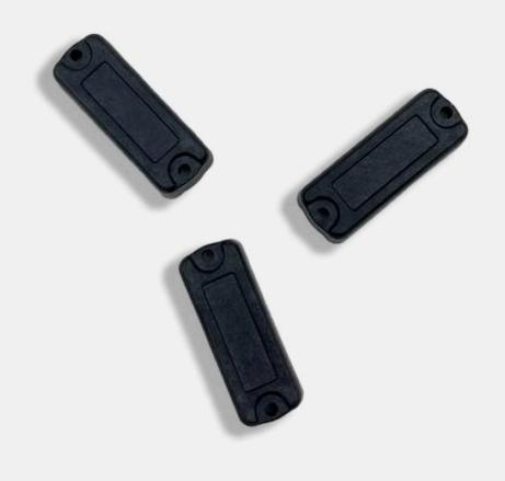
HT009 is an RFID tag made of PPS, a material that is **resistant to very high temperatures** - up to 260°C for 30 minutes and 180°C for 120 minutes - and **can be applied to metal surfaces**.
