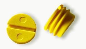
HT017 is an RFID hard tag made of nylon, ultra light material fiber, which responds well to damage due to wear, traction, chemical agents, mold and bacteria. Designed to be incorporated into metal surfaces, its shape is cylindrical, it is ultra light it weighs only 0.25 grams! - with a diameter of 6.8 mm and a height of **4 mm.** Available in yellow, this tag is personalised through laserization. In addition, the HT017 hard tag is equipped with ICODE SLIX2 chip, with HF frequency, at 13.56 MHz.
