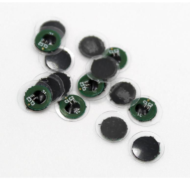
HT021 is a 'PCB tag' comprising a printed circuit board (PCB) substrate, an insulating printed circuit board that connects several electronic components, protected by fibreglass. This layer is covered by thin metal applied via high-temperature rolling. Finally, the tag surface features a thin polycarbonate plate.
