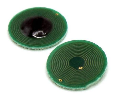
HT020 is a 'PCB tag' featuring a PCB (printed circuit board) substrate, an insulating printed circuit board that connects various electronic components. It is protected by a *fibreglass* plate covered with a light layer of metal applied using high-temperature pressing following the lamination process.
