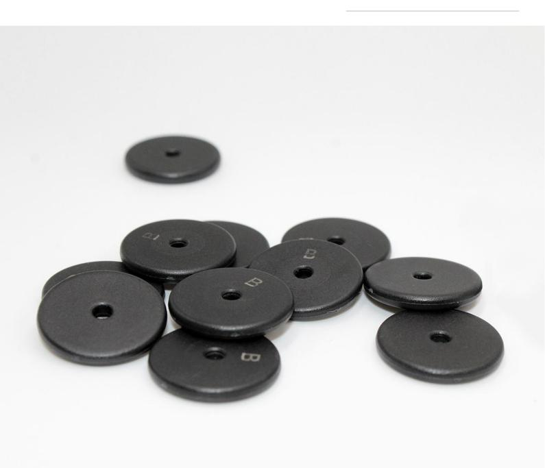
HT022 is an RFID hard tag made of PA9T nylon resin, a special polyphthalamide with outstanding properties in terms of dimensional stability, fluidity and thermal, chemical and abrasion resistance. Round in shape, it has a slim but robust housing. With a 22-mm diameter, 3-mm thickness, and 3.1-mm central hole, HT022 is
