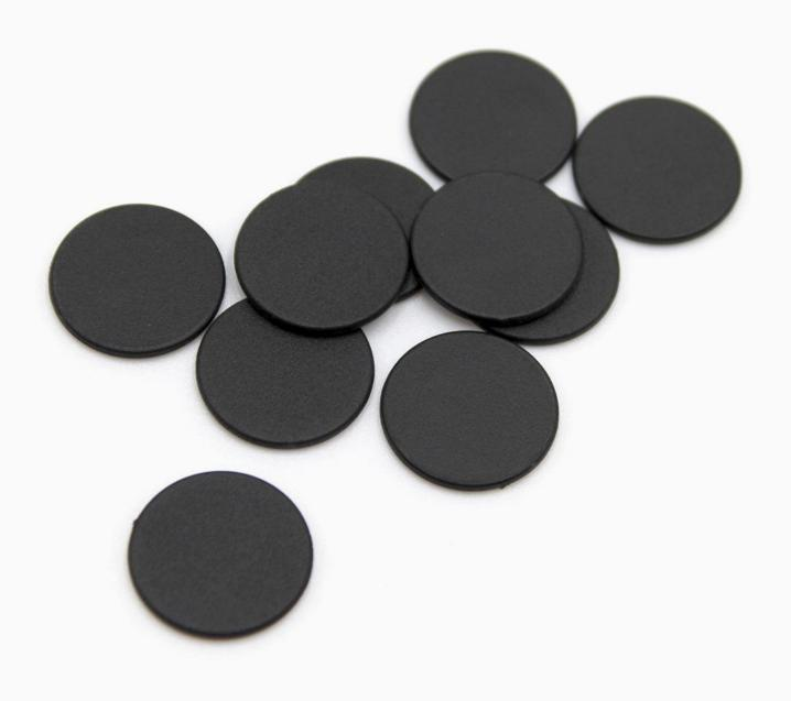
HT025 is a 'button tag' made of nylon, a material that is both thin and strong, while offering high resistance to impacts, chemicals and bacteria. Round, ultra thin and ultra small — 16.2 mm in diameter, 1.35 mm thick and weighing just 0.3 grams — this RFID tag is designed for application on small, non-metal objects using an adhesive backing.
