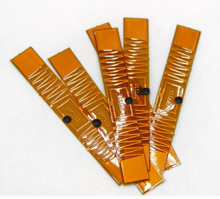
HT032 is a 'mould tag', a special RFID tag that is embedded into the product via injection moulding during production. It is made of FPC (flexible printed circuit), a printed circuit consisting of a polyamide or polyester film which is extremely light, thin and flexible. Yellow in colour and rectangular in shape, it measures 70 mm x 11 mm x 0.6 mm. Weighing just 0.2 grams, it is
