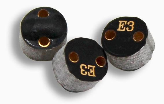
HT060 is an RFID hard tag made of FR4 (flame resistant), a material made of fibreglass with an epoxy resin matrix, which makes it **flame retardant**. It has a high electrical resistance and very low degree of moisture absorption.
