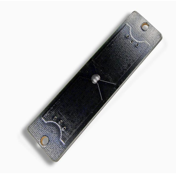
HT061 is an RFID hard tag made of FR4 (flame resistant), a material consisting essentially of fibreglass and a flame-retardant epoxy resin. With high electrical resistance, this material absorbs very little moisture. It is also resistant to acids and alkaline substances.
