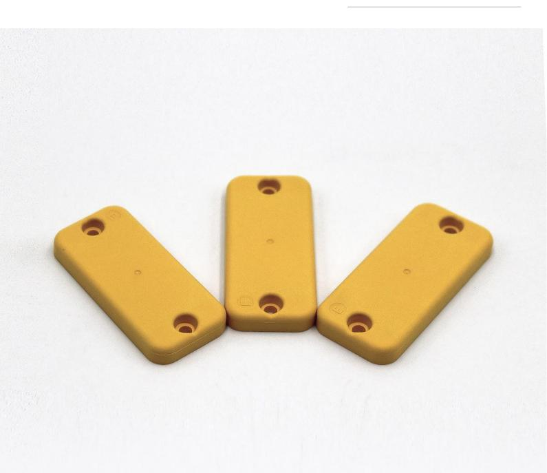
HT064 is a nylon RFID hard tag resistant to impacts, tensile stress and chemicals. Rectangular in shape - measuring 52 mm x 23 mm x 5.5 mm and weighing 11 grams - this robust RFID tag optimised reading guarantees performance in metal-dense environments. It is resistant to verv high temperatures, with a maximum temperature of +200°C for one hour. HT064 is particularly designed
