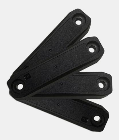
HT071 is an RFID hard tag made of nylon, a material which gives rigidity, compressive strength and dimensional stability. Rectangular in shape - measuring 78 x 21 x 11 mm - this robust RFID tag is designed to be applied to even narrow metal objects by screwing.
