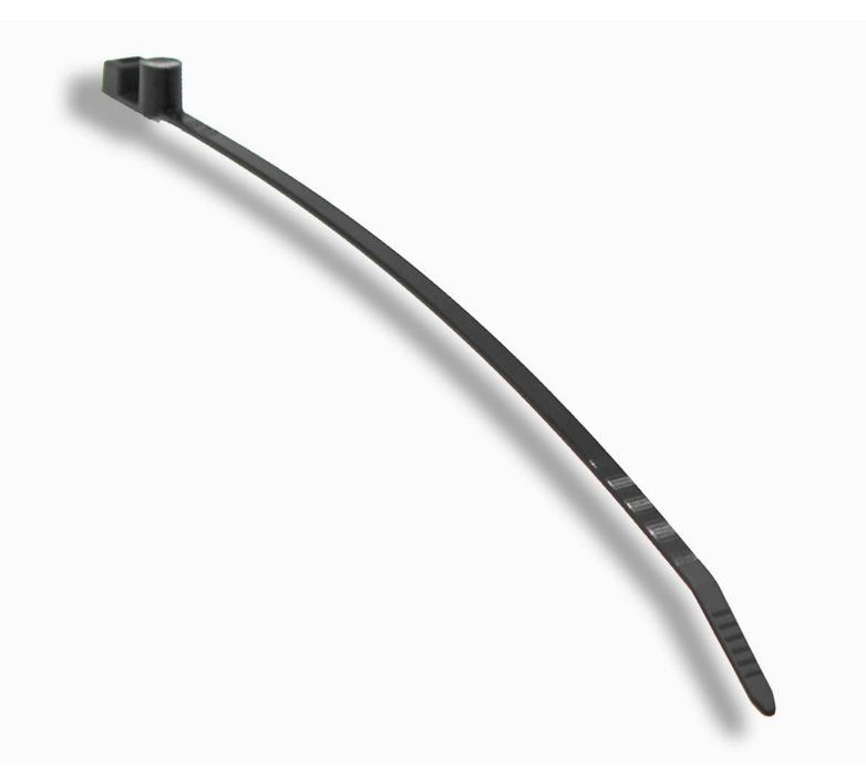
HT083 is a **cable tie tag** made of PA66, a nylon featuring hardness, rigidity and resistance to wear, heat and abrasion. It measures 198.5 mm x 9 mm x 8 mm and weighs 2 grams. With its special cable tie shape, it can be firmly anchored to **objects for identification purposes**. Designed for application on non-metal surfaces, HT083 is
