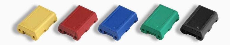
HT085 is a 'sleeve tag' or 'tag anchored to objects using a cable tie' made of PA6, ultrasound-sealed nylon that provides good thermal protection and perfect resistance to impacts, pressure and other mechanical stresses. Rectangular in shape - 27 mm x 20.7 mm x 9.6 mm - and weighing 4.7 grams, this tag can be anchored to metal surfaces by means of plastic or metal cable ties. It is available in LF with the
