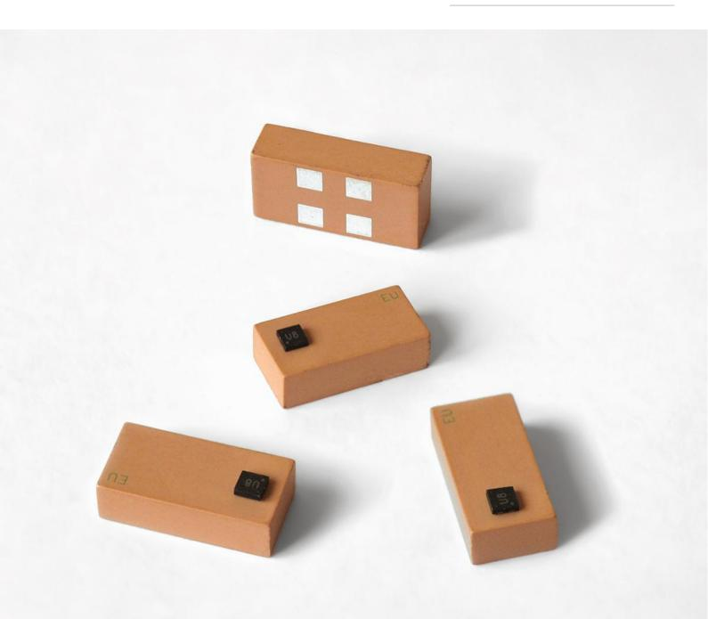
HT086 is a hard **ceramic tag** featuring low electrical conductivity and resistance to high temperatures. Rectangular, small and thin – measuring 10 mm x 5 mm x 3 mm – it is **ideal for small spaces and can be glued to the surface of metal objects.** HT086 is yellow and available in **European** and US UHF with the UCODE 8 chip.
