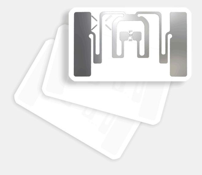
LB014 is an RFID label made of PET, a flexible, cut- and weather-resistant thermoplastic material. It is rectangular and measures 54 mm x 34 mm x 0.24 mm. LB014 can be applied to non-metal surfaces using a special adhesive. Printing and serial numbering are applied using offset or inkjet technology for colour and black-and-white prints, and thermographic printing for black and white only. White in
