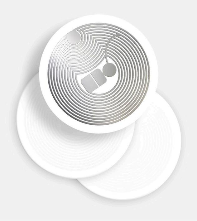
LB016 is a flexible and adhesive RFID label made of coated paper. Round in shape, it has a diameter of 17 mm, while the engraved aluminium inlay or antenna has a diameter of 15 mm. It can be applied to non-metal surfaces and resists at high temperatures of up to 80°C during operation. It can be customised using offset or inkjet technology in colour and black and white, and thermographic printing in
