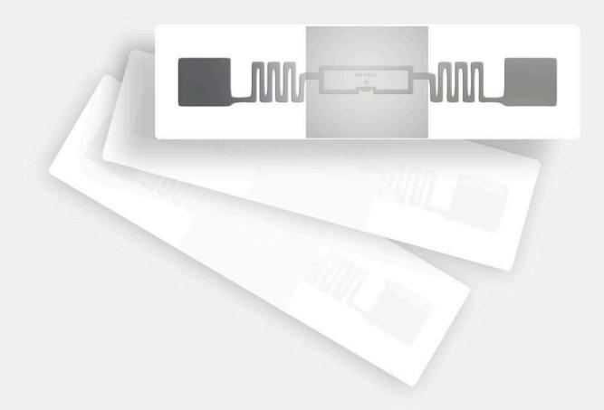
LB020 is an RFID tag made of PET, a flexible thermoplastic material resistant that is to cuts, atmospheric changes and high temperatures. Indeed, this label can tolerate up to 70°C in operation and storage. Rectangular in shape, it measures 106.5 mm x 28.5 mm; the antenna has the following dimensions: 95 mm x 12 mm. LB020 is applied to non-metal materials by means of an adhesive
